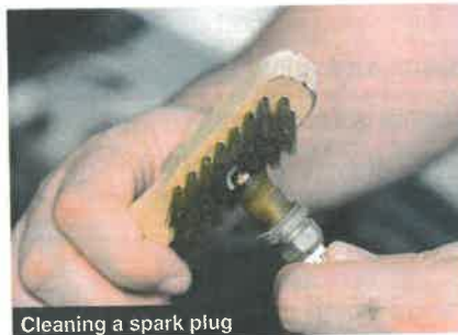
Cleaning a spark plug
